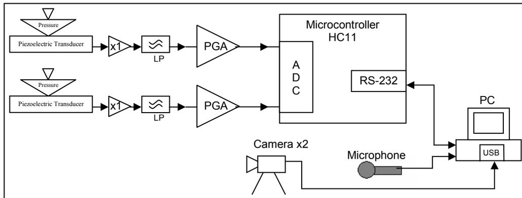
Figure 1. Connection of the hardware used for the footstep capture system.
