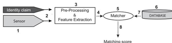
Figure 1: Architecture of an automated biometric verification system, with the possible points of attack identified in [20].
