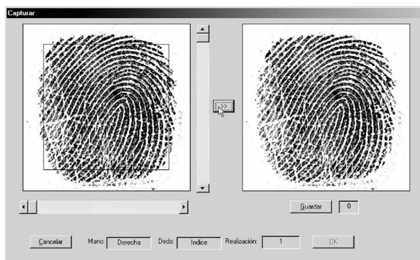
Fig. 1 Acquisition interface for the CMOS capacitive device
