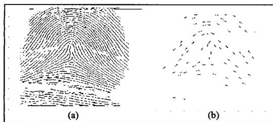
Figure 6: (a) Image after thinning and imperfection removal. (b) Minutiae pattern after cluster elimination process.
