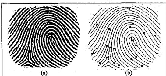
Figure 9: (a) Original fingerprint. (b) Detected minutiae.
