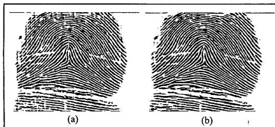
Figure 5: (a) Image after the first profiling filtering. (b) Image after the second profiling filtering with spatial mask.
